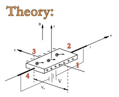
Let us consider a P-Type semiconductor Sample placed in a magnetic field as shown in the figure,
